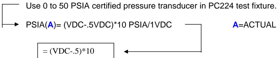
Note: Open the PC224 test unit pressure transducer to ambient.
