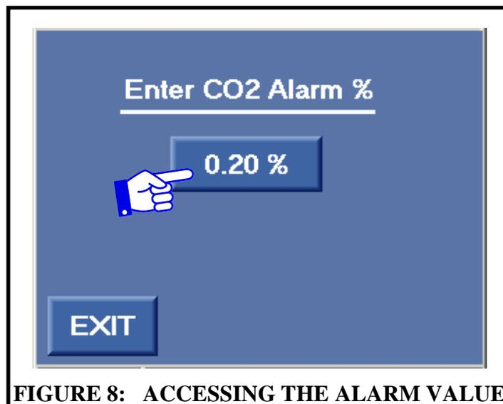
Pressing the button shown in figure 8 will cause the virtual keypad in figure 9 to appear. The factory default for the alarm is .2%, but it can be adjusted from zero to .50% in .01% increments. This setting is an absolute value. If the value is set for .2%, the alarm will turn on if the actual concentration calculated from the flow meter feedbacks is outside the range of 4.8% to 5.2%. Simply enter the error value and press the enter key.
