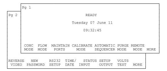
The instrument was designed with emphasis on simplicity and ease of use. The menu driven software guides users through all operating routines and provides on-screen mode specific help with the simple press of the "help" key. The main menu offers 13 primary options; each is described briefly below:
